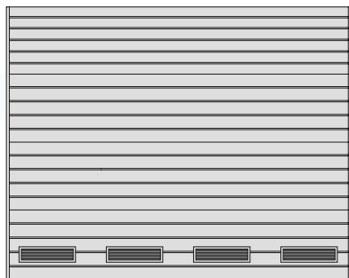
GARAGE DOOR WITH VENTILATION GRILLES
