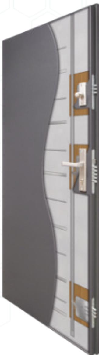
47 MM THICK LEAF WITH A THREE-SIDED UPSTRAND, MADE OF 1.2MM GALVANIZED AND LAMINATED SHEET, FILLED WITH FOAMED POLYSTYRENE [STYROFOAM], EQUIPPED WITH A GASKET
